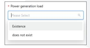
• Set system parameters to ensure normal reading of electrical parameters in AC Couple mode, specifically under the "Power generation load" entry. (This parameter is only supported by Solarman Business.)
